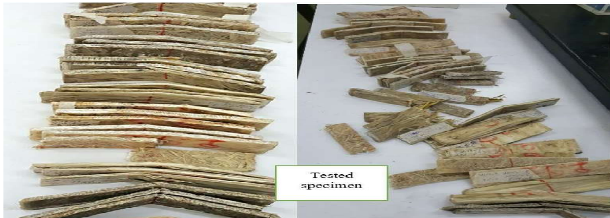
Fig.10. Specimen after flexural strength test
