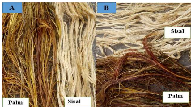
Fig.6. Treated fiber after dried in sunlight; A , treated with 6%,NaOH, B , treated with 10%NaOH. The surface of the fiber was changed its color and morphology after NaOH solution treatment in different concentration.
