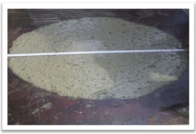
Fig.-4.2 T50cmFlow Test
