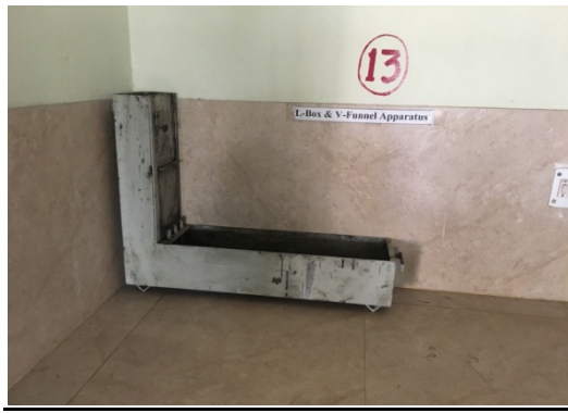
Fig.-4.4 L-box apparatus and its dimensions
