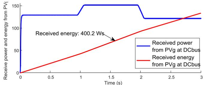
Fig. 13 Power and energy received at DCbus
