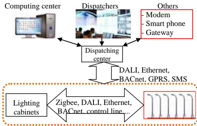
Fig. 8 Architecture of control and data acquisition applied in street lighting systems
