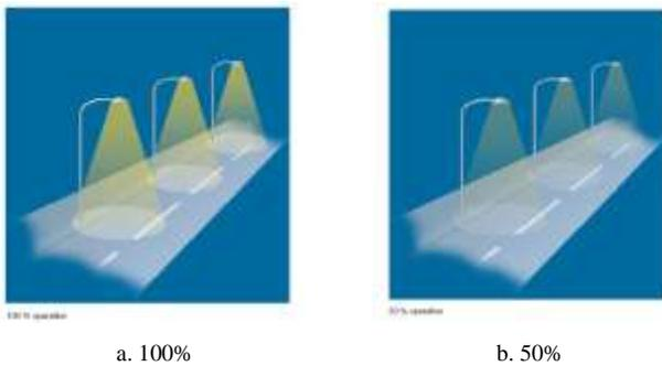
Fig. 6 Decrease the brightness of luminaries using dimmers
