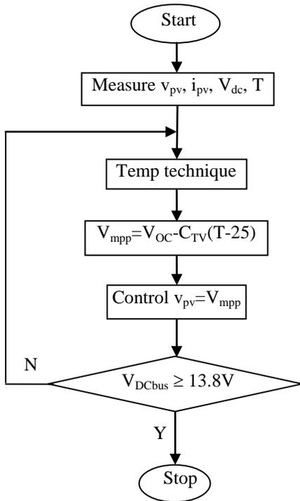
Fig. 10 Algorithm to harness energy from PVg and charge energy to battery
