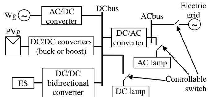
Fig. 8 Hybrid structure harnessing PVg and Wg
