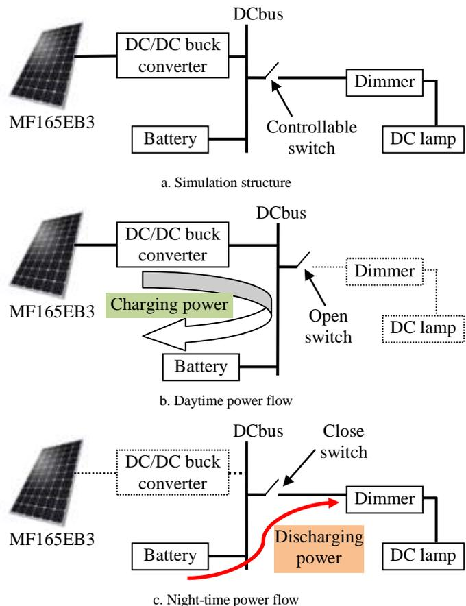
Fig. 9 Structure and power flow in simulation system
