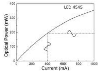
Fig. 4 Power - current characteristic of LED lamp
