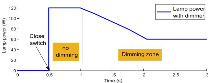
Fig. 15 Power consumed by DC lamp with dimmer
