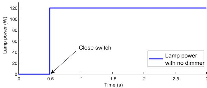
Fig. 14 Power consumed by DC lamp with no dimmer
