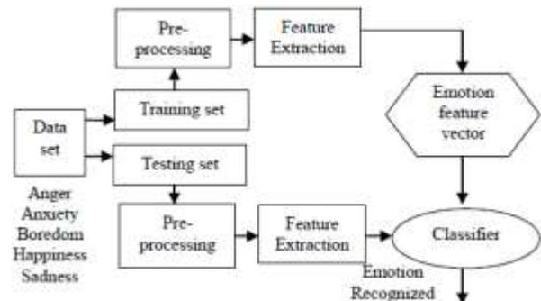
Fig 1. Steps in Training and testing the emotion recognition system.
