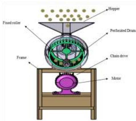
Figure 6: Perforated drum and stationary roller sorghum peeler
