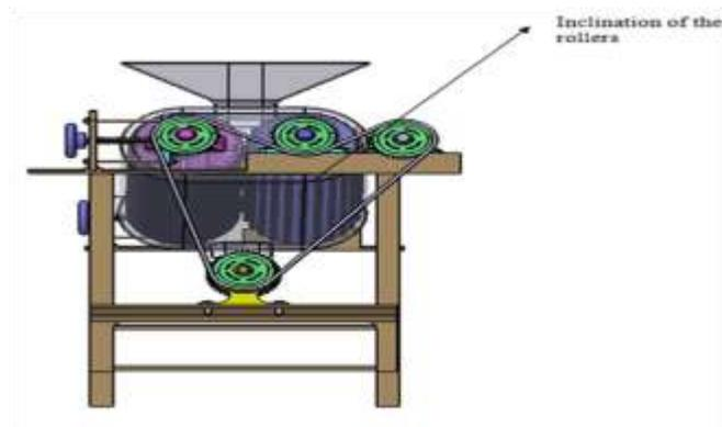
Figure 5: Abrasive Drum and Brush roller Sorghum peeler
