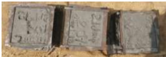
Fig 3 Casting of Cubes
