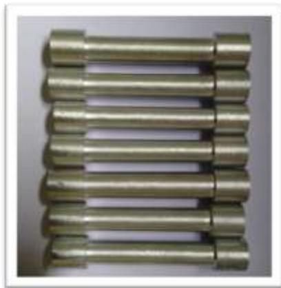
Figure 6: Tensile test specimens
