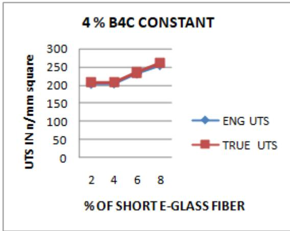
Figure 8: UTS (Mpa) v/s varying % of short E-glass fiber (4% B4C constant)
