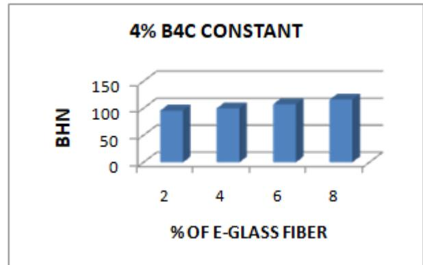
Figure 12: Hardness v/s varying % of short E-glass fiber (4% B4C constant)
