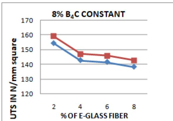
Figure 10: UTS (Mpa) v/s varying % of E-glass fiber (8% B4C constant)
