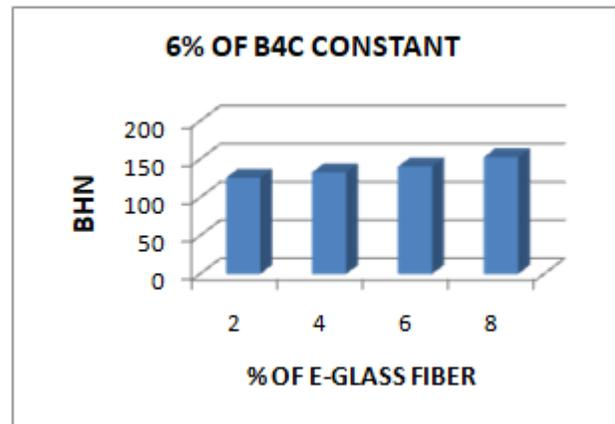
Figure 13: Hardness v/s varying % of short E-glass fiber (6% B4C constant)
