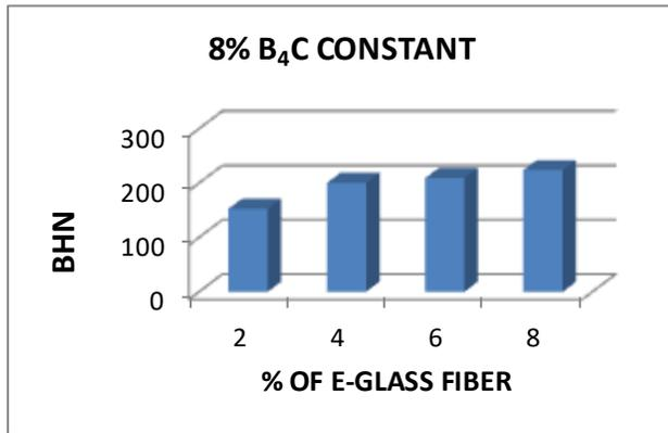
Figure 14: Hardness v/s varying % of short E-glass fiber (8% B4C constant)
