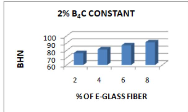
Figure 11: Hardness v/s varying % of short E-glass fiber (2% B4C constant)
