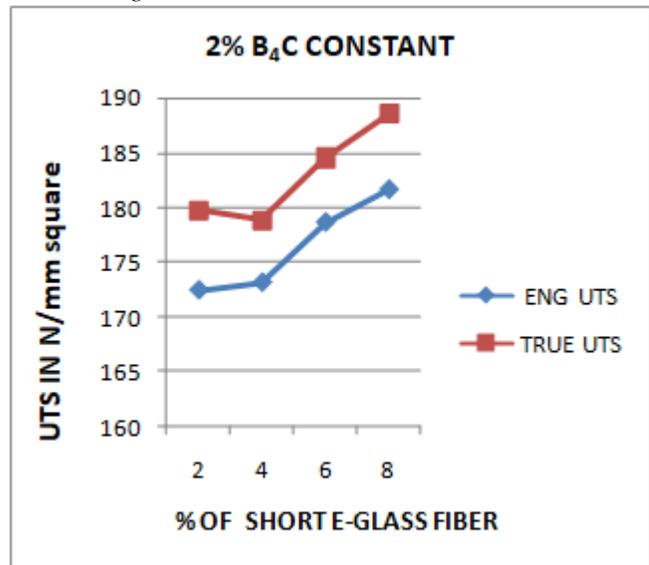
Figure 7: UTS (Mpa) v/s varying % of short E-glass fiber B4C constant)
