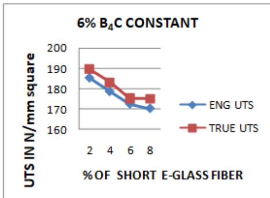
Figure 9: UTS (Mpa) v/s varying % of E-glass fiber (6% B4C constant)
