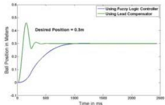
Fig..10. Output response-2 of the DMBB system using various Controllers
