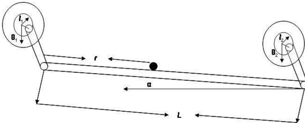
Fig. 4. Kinematics diagram of DMBB System
