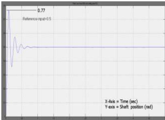
Fig. 7. Response with 50% Peak over shoot and 0.5s settling time
