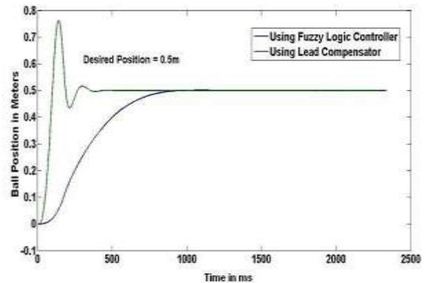
Fig..9 Output response-1 of the DMBB system using various Controllers
