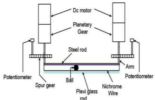
Fig. 1. Top view of the DMBB system
