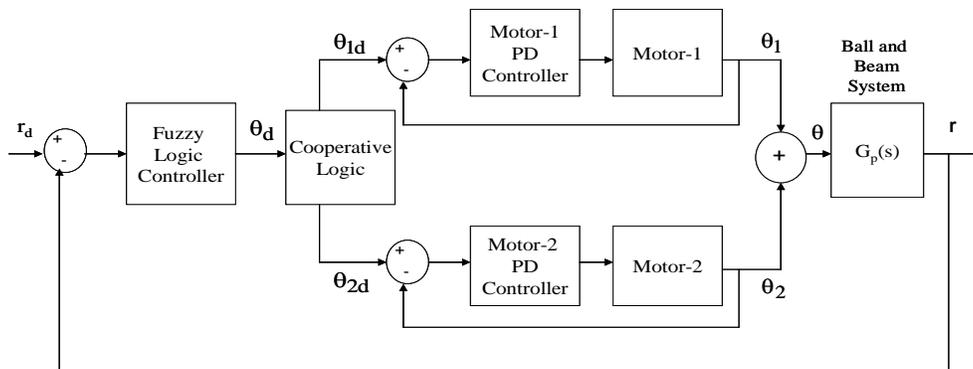
Fig. 6. Block diagram of closed loop control of DMBB system
