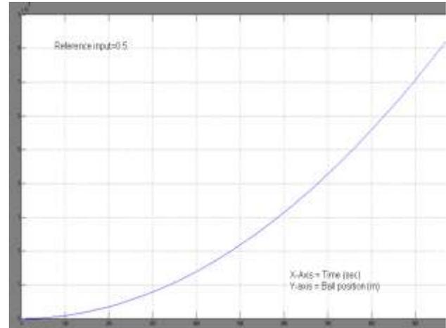
Fig. 5. Open loop Step Response of DMBB System
