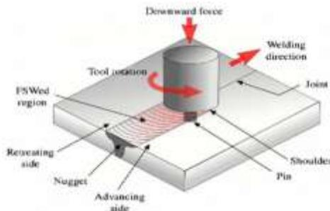
Fig. 2 Welding process
