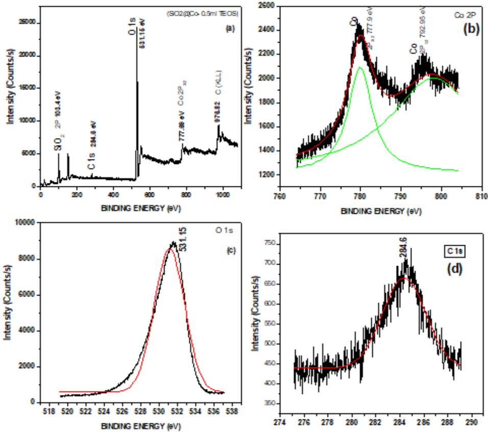
**Figure 4.1** XPS spectral line fit (a), Co@SiO<sub>2</sub> Core/Shell (0.5 ml TEOS coated) nanoparticles wide range spectrum (b), Co 2p spectrum (c), O(1s) spectrum and (d) Internal reference C(1s) spectrum. Hint: The spectral curve fitting was performed with OMICRON CASAXPS software version 2.3.
