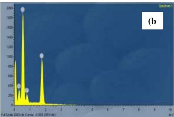
Figure 3 EDAX spectrum of (a) 0.5 ml TEOS, (b) 1ml TEOS coated core- shell
