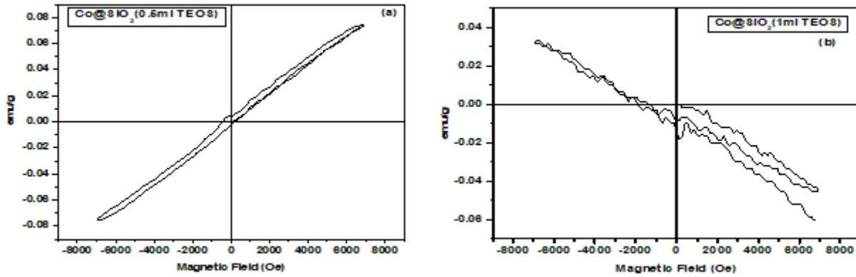
Fig.5. Hysteresis loop for (a) Co@SiO<sub>2</sub> core-shell (0.5 ml of TEOS, annealed at 500°C for 19 h), (b) Co@SiO<sub>2</sub> core-shell (1 ml of TEOS, annealed at 500°C for 19 h, samples measured at 300°K.
