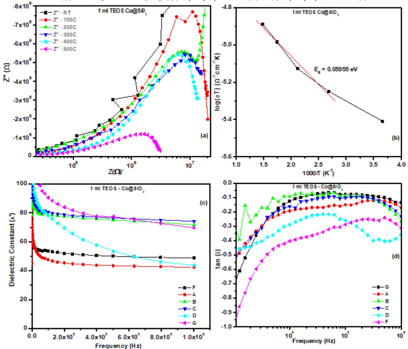
Fig.7. Impedance plots at high temperatures for nanocrystalline Co@SiO<sub>2</sub> (1 ml TEOS-coated Co) core/shell sample annealed at 500°C for 19 h (a) RT – 500°C, (b) Arrhenius plot of Co@SiO<sub>2</sub>, (c) frequency dependence of ( $\epsilon'$ ) and (d) frequency dependence of  $\tan(\delta)$ .
