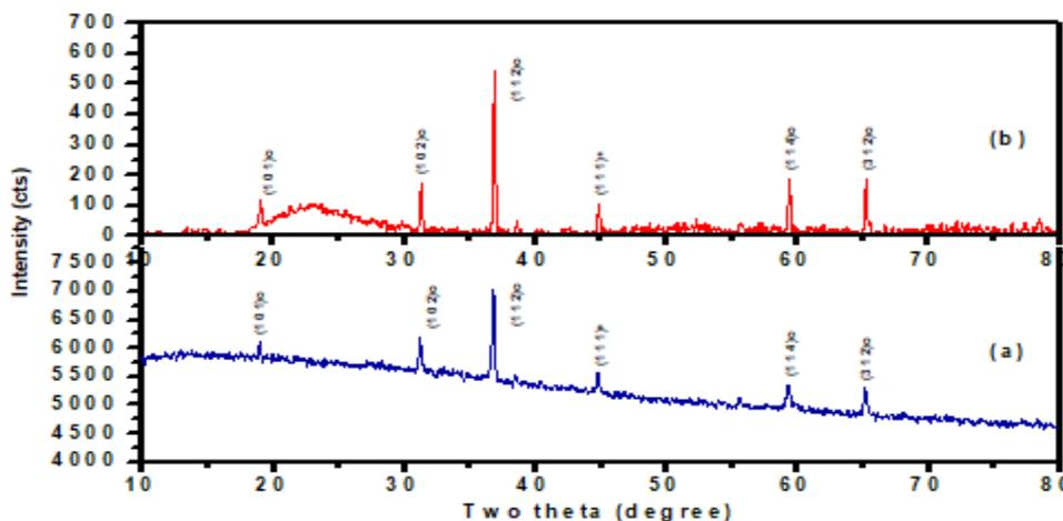
**Figure 1** X-ray diffraction results for  $Co@SiO_2$  annealed at  $500^\circ C$  for 19 h samples. (a) 0.5 ml of TEOS concentration, (b) 1 ml of TEOS concentration, annealed at  $500^\circ C$  for 19 h, (\*, °) Star represent cobalt peak, and open circle represent  $SiO_2$  peak
