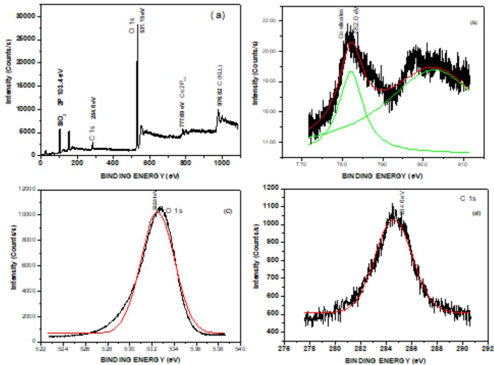
**Figure 4.2.** XPS spectral line fit (a), Co@SiO<sub>2</sub> Core/Shell (1 ml TEOS coated) nanoparticles wide range spectrum, (b) Co 2p spectrum, (c) O(1s) spectrum, and (d) Internal reference C(1s) spectrum. The spectral curve fitting was performed with OMICRON CASAXPS software version 2.3.
