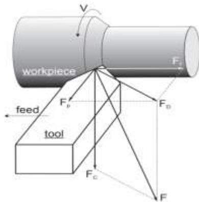
Fig. 2 Force components in three-dimensional oblique cutting
