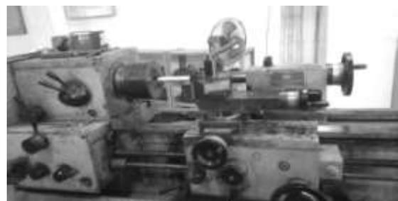
Fig. 3 Lathe with dynamometer
