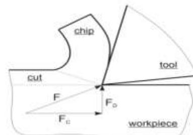
Fig. 1 Schematic view of Orthogonal Cutting Force
