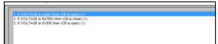
Fig. 9. If-then rules used for mapping the input mf to the output mf.
