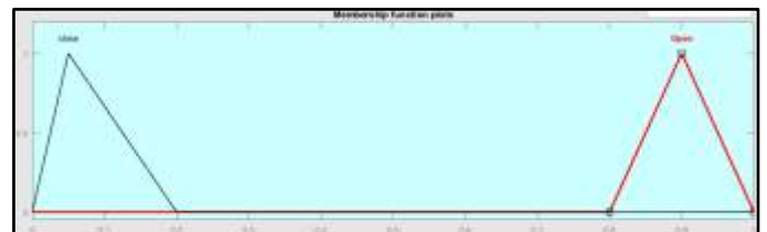
Fig. 5. Membership function for second output to switching the motor OFF.
