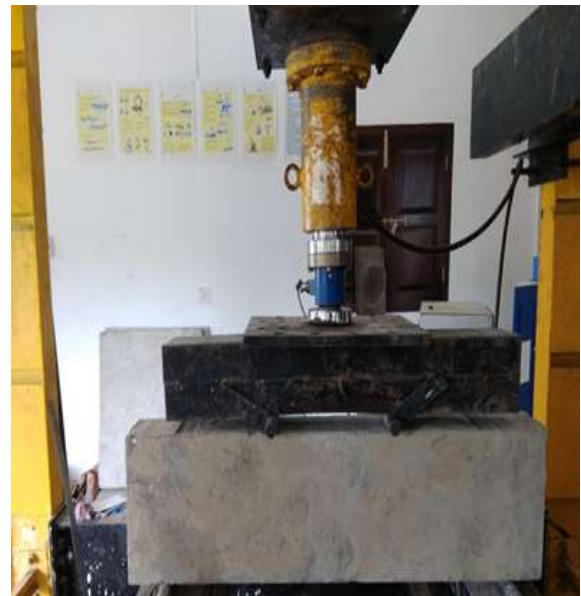
Fig 10. Test setup of flexural loading beam
