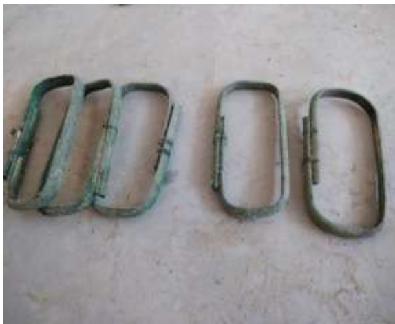
Fig 9. Coated bamboo reinforcement
