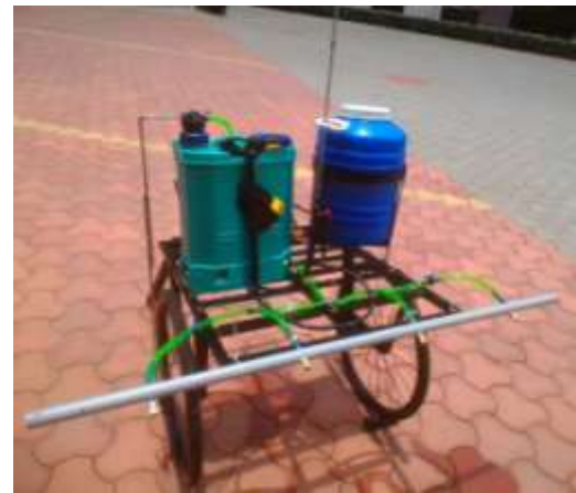
Figure 4.2: Actual model of multipurpose pest sprayer
