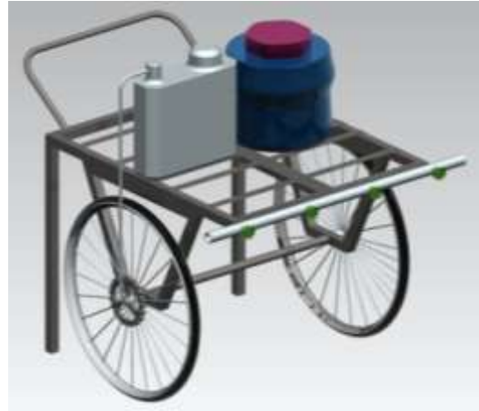
Figure 4.1: CAD model of multipurpose pest sprayer
