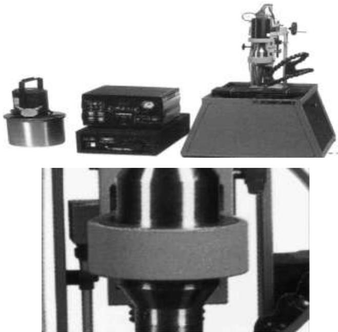
Fig. 3. Compact 500W USM machine for small, light-weight work piece [9].
