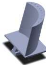
Fig3. Turbine second stage rotor blade with 9 holes
