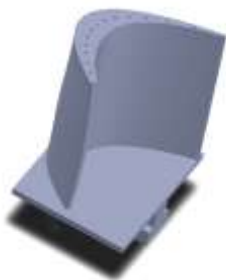
Fig4. Turbine second stage rotor blade with 13 holes
