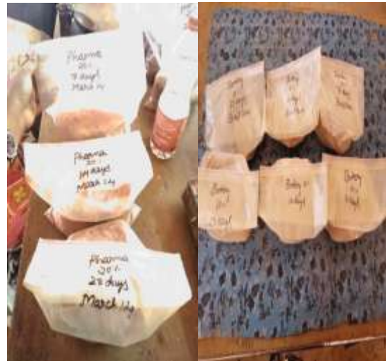
Figure 1: Contaminated soil kept for curing in air tight containers
