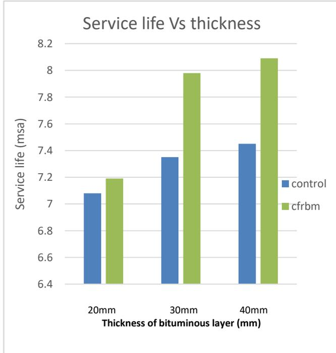
Fig.5. Service life of pavement sections in fatigue
