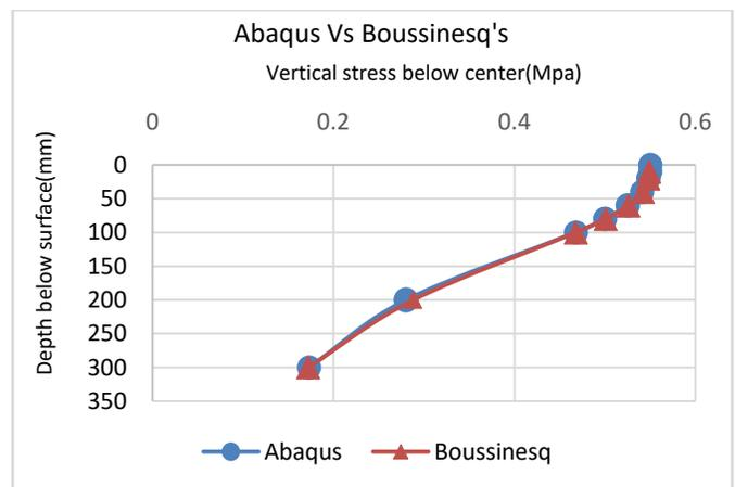
Fig.3 .Validation of Finite element analysis
