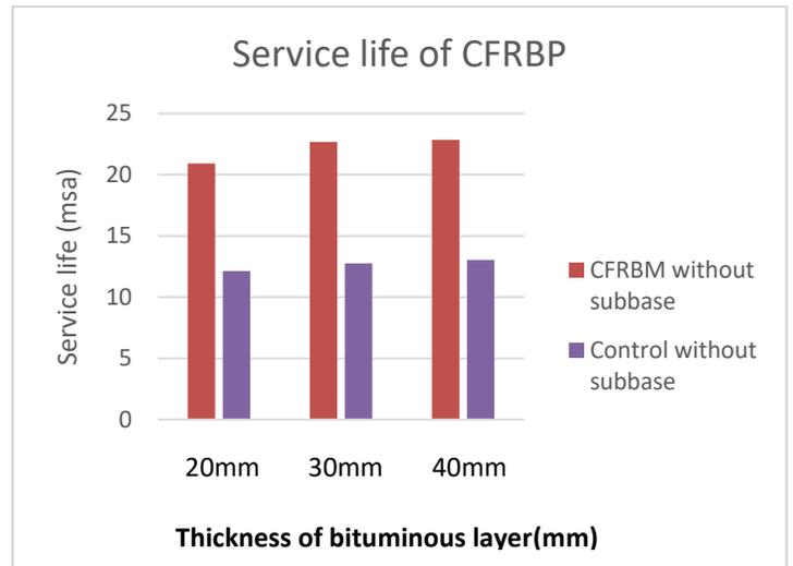
Fig.6 . Service life of pavements in rutting
