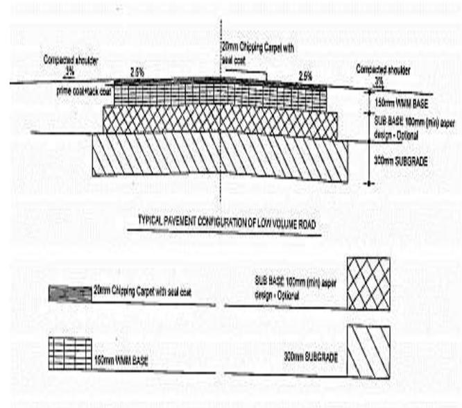
Fig.1. Typical Pavement Configuration of Low Volume Roads (source IRC SP 72-2015)
