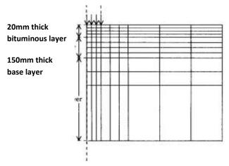
Fig2. Finite Element Model
