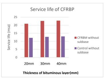
Fig.6. Service life of pavements in rutting
