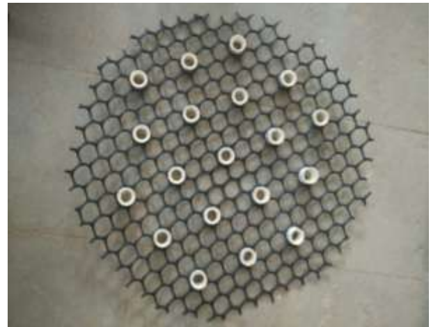
Fig 1: Layer of Geogrid-PVC Pipe
