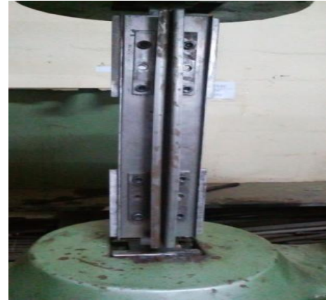
Fig.9 Angles fixed in universal testing machine (UTM)
