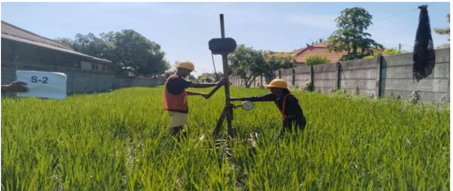
Figure 2. Illustration of manual cone penetration test using manpower
