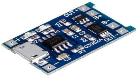
Figure3: TP4056 Charging Circuit
