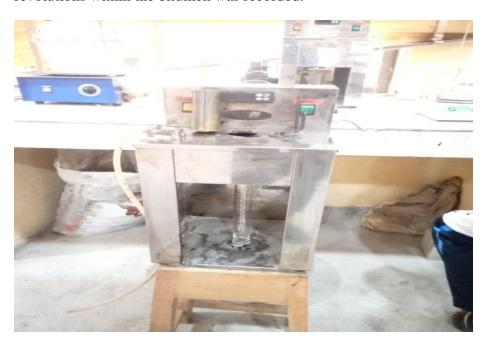
**Typical Rotational Viscometer**
