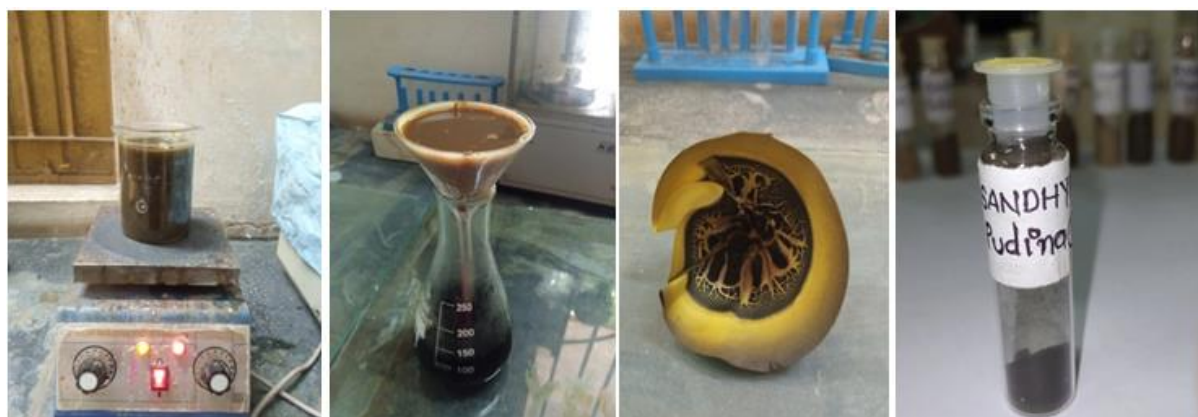
Figure 3: FeO Solution Using Pudina Leaf Extract (a) While Stirring (b) While Filtration (c) After Filtration (d) After Calcination.
