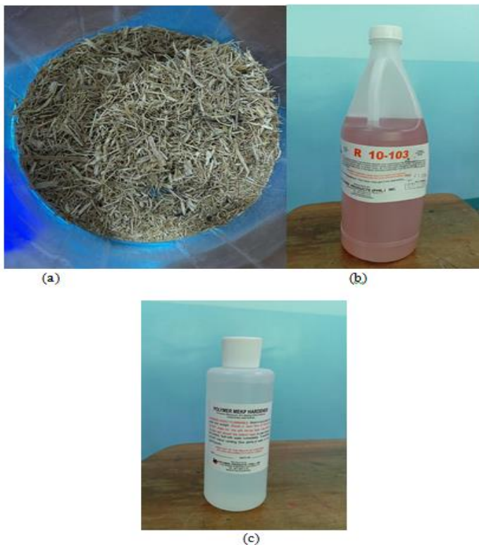
Fig 2. Photo samples of (a) sugarcane bagasse fibers, (b) polyester resin, and (c) polymer hardener
