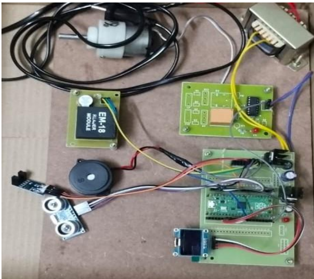
Fig 2: Simulation and results of Anti-Collision Speed Control System Based on Embedded System Using RFID
