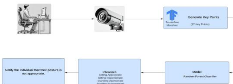
Figure 1: AI-powered pipeline for posture detection, integrating TensorFlow MoveNet for key point extraction and machine learning classifiers for posture categorization."
