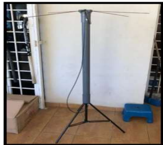
Figure 3. Construction of the cross-dipole antenna, showing the copper rods and PVC mounting
