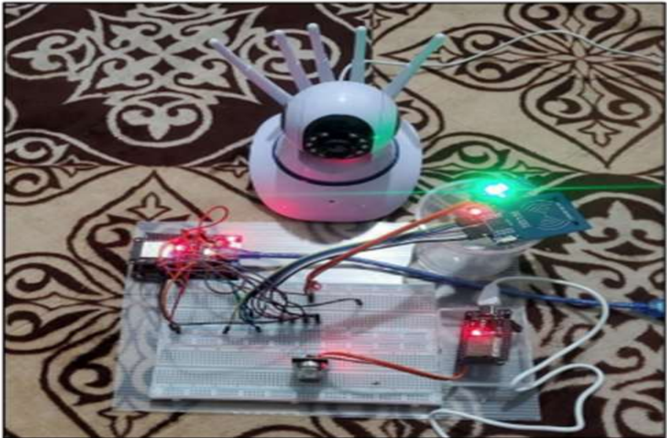
Fig. 7 Successful Connectivity NodeMCU and RFID Sensor.
