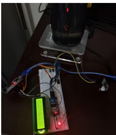
Figure 24: Breadboard Development of the IoT-Monitored Oil Collecting System Used for Early Validation of Sensing, Display, and Connectivity
