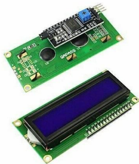
Figure 18: Assembled 16×2 LCD with I 2 C Interface as Implemented in the Prototype
