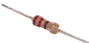
Figure 20: 220 \Omega Fixed Resistor Used for LED Current Limiting in The Prototype
