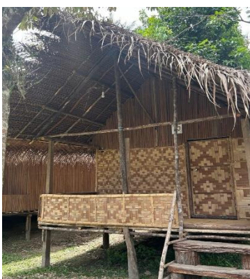
Figure 4: Chalet Gepeh (wall made from kelarai bertam)
