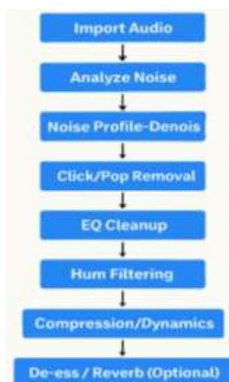
Figure 4. Technical Process of audio restoration in FL STUDIO
