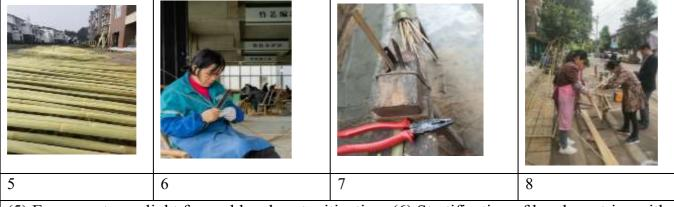
(5) Exposure to sunlight for mold and pest mitigation; (6) Stratification of bamboo strips with selection and retention of outer layers; (7) Subsequent subdivision of bamboo strips for desired dimensions, ensuring uniform width; (8) Implementation of weaving on metallic templates
