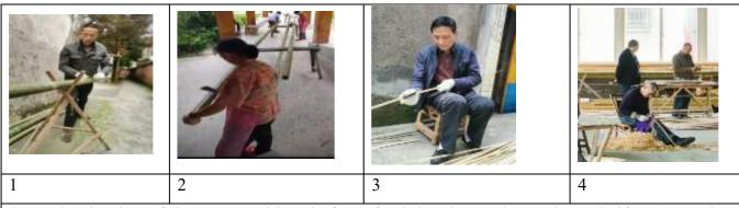
(1) Delaminating of the green epidermis from fresh bamboo culms using a knife; (2) Cutting of bamboo culms to specified lengths, smoothing saw kerfs; (3) Uniform splitting of bamboo culms into segments of equal size; (4) Abrasion and refinement of bamboo strips to achieve desired thinness;
