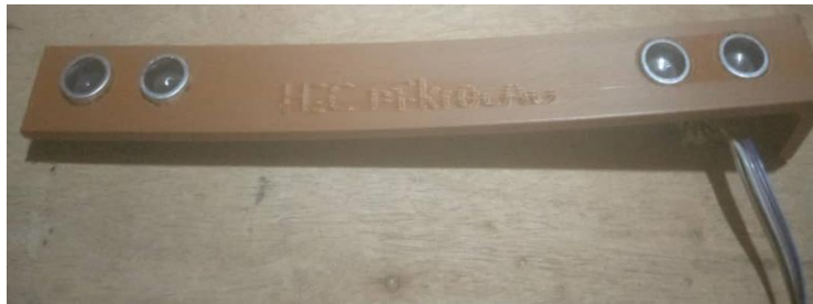
Fig. 7(a): Sensor showing the transmitter and receiver
