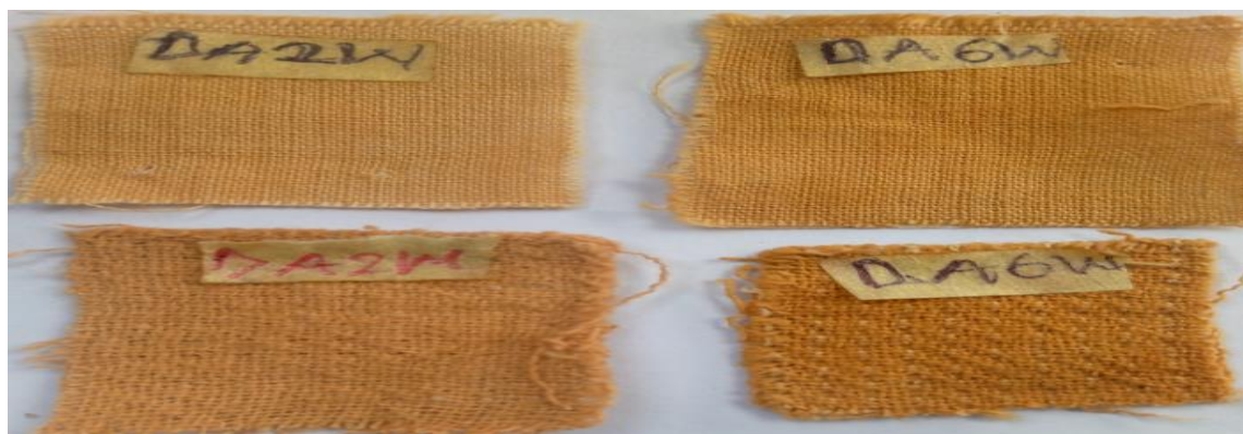
Fig 6: Cotton and wool fabrics dyed with dye extract and tested for wash fastness
