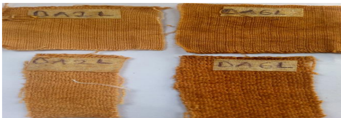
Fig 8: Cotton and wool fabrics dyed with dye extract and tested for light fastness
