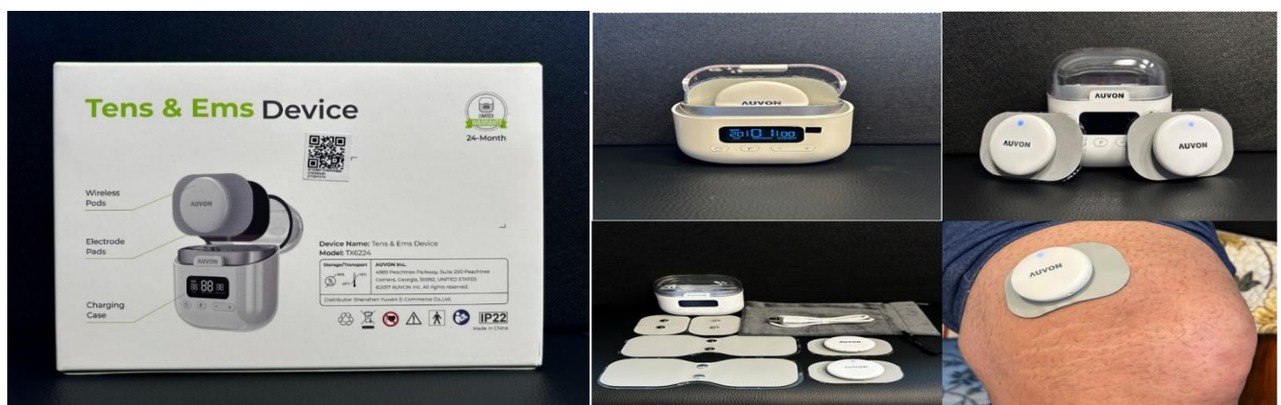
Figure 5. various views and components of the TENS & EMS Device, including its packaging, the main unit in its charging case, detached electrode pads, and all accessories.
