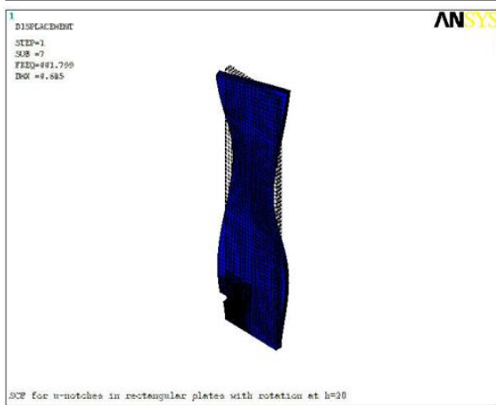
Figure 7: 2T mode of rectangular blade with semicircular notch at h = 20\text{mm}
