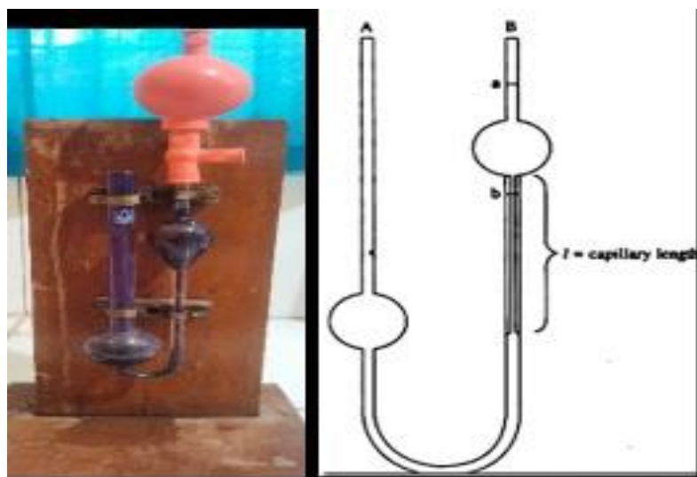
Figure 3. a) Ostwald viscometer b) Sketch of Ostwald viscometer section
