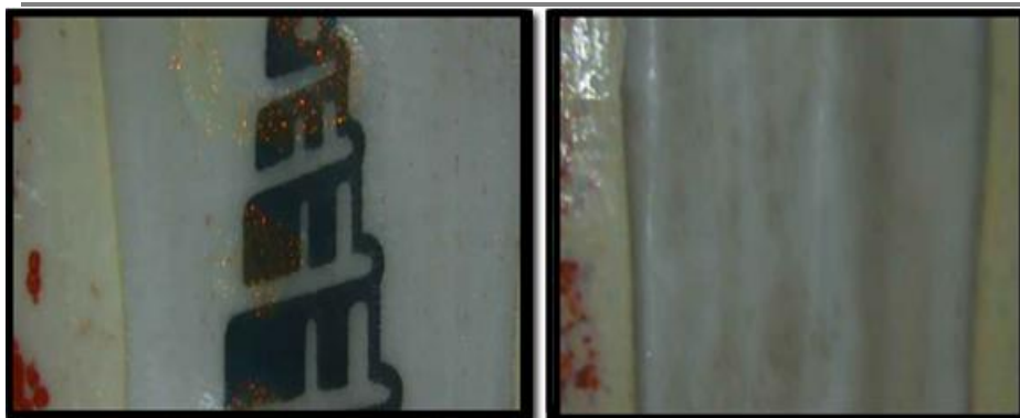
Figure (6) shows a microscopic image of the original (left) and counterfeit (right) 25000 class transparent window.
