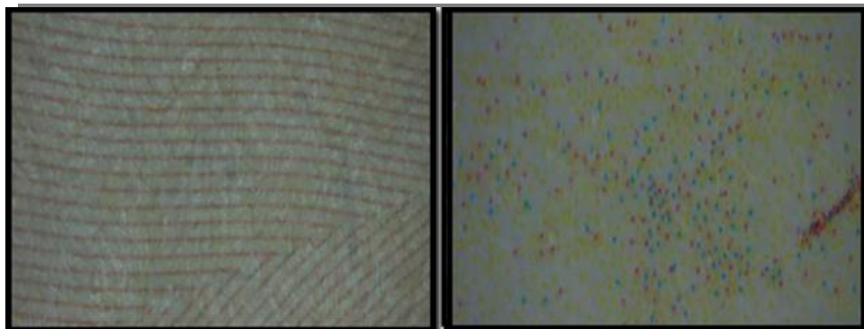
Figure (10) shows an under-microscope image of the 10,000 class of the original (left) and Counterfeit (right) watermark.
