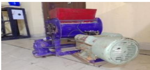
Fig. 14 Electric motor attached to the machine
