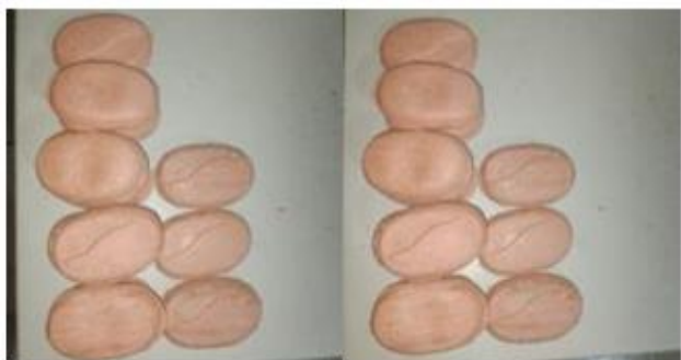
Fig. 16 Bar soap produced using the triple roll mill
