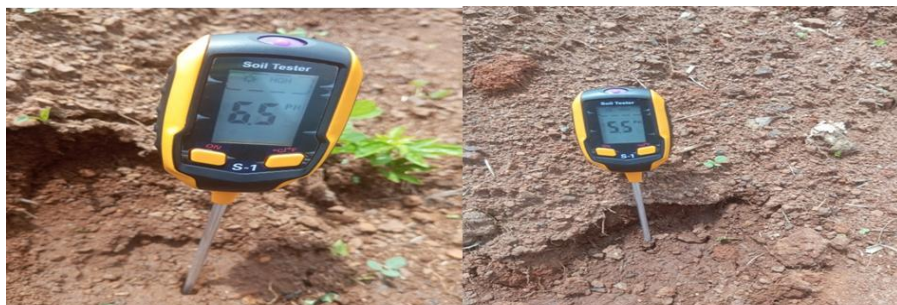
Fig. 2: Soil pH tester displaying reading on site
