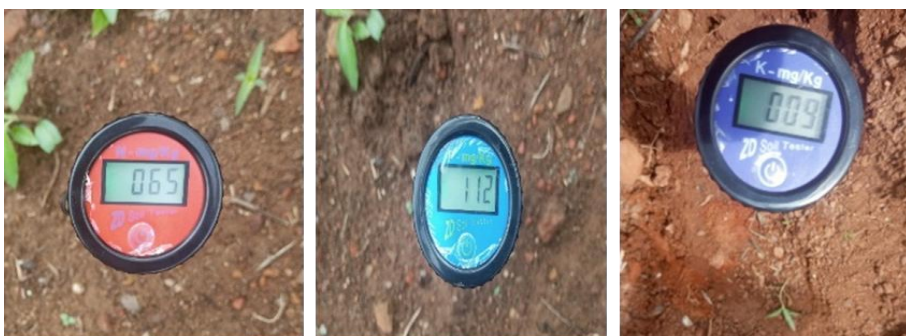
Fig 4: On-site reading of the NPK meter
