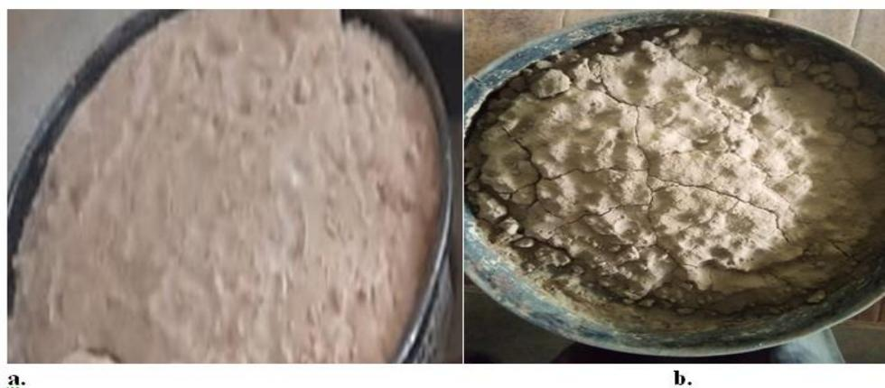
Plate II: Crust thickness: (a) natural with no crust (powdery form) (b) bio-treated soil with crust thickness formed before wind-induced load
