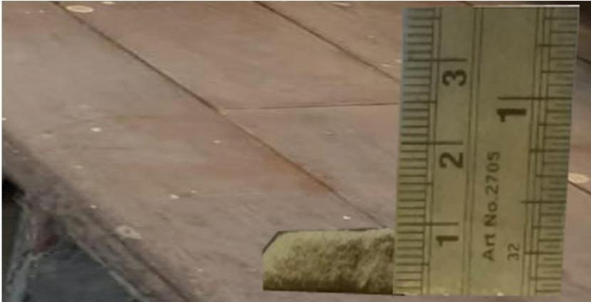
Plate IV: Soil crust thickness of bio-treated aeolian soil sample treated for higher wind speed of 20 m/s at  $6 \times 10^8$  cells/ml – 0.75 M.
