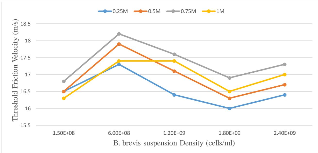
Figure 2: Variation of the TFV of the aeolian soil with *B. brevis* suspension density and cementation reagent treatment at 20 m/s wind speed
