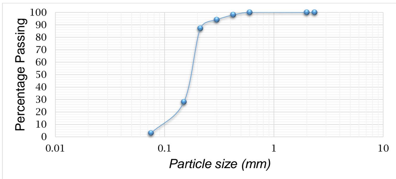
Figure 1: Particle size distribution curve for the natural aeolian soil.
