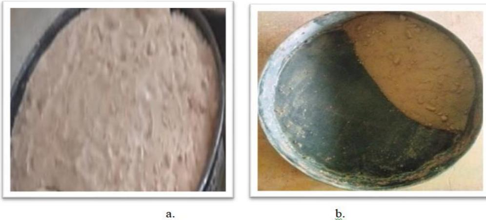
Plate I: Natural soil sample (a) before and (b) after experiencing wind load.
