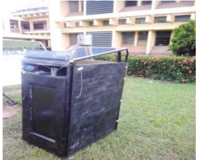
Fig. 1 picture of the solar thermal clothes drying system.
