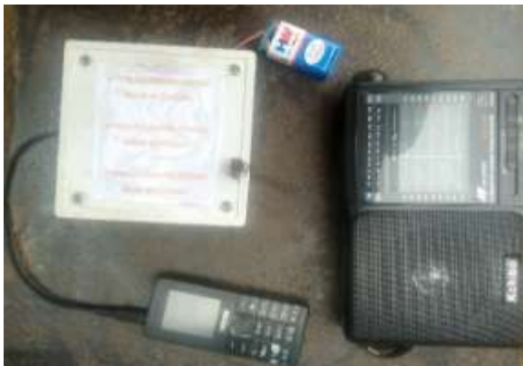
Figure 3: JP Low Cost Wireless Public Address System.
