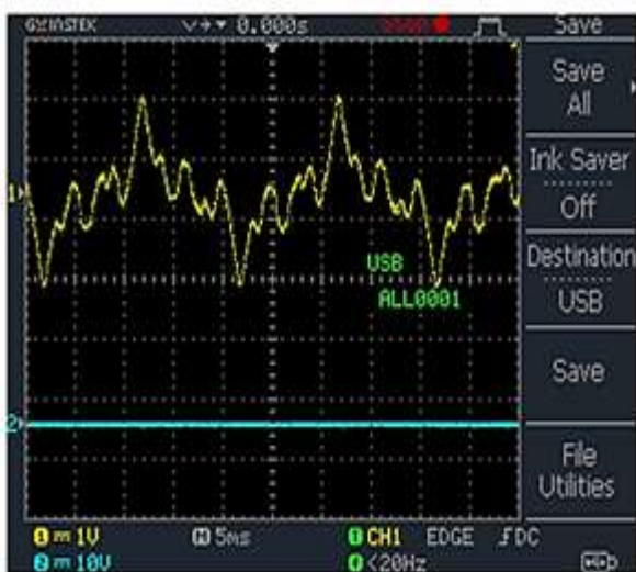
Figure 9. CVT Input Voltage Waveform on Storage Screen Oscilloscope with 1.5 kW Heater Element Connected
