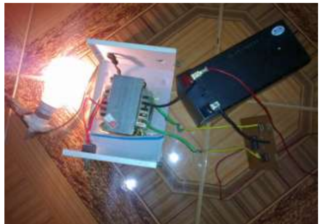
Fig. 6: Tested and Verified Inverter Circuit
