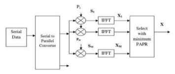
Fig.2. Block diagram of Selective Level Mapping
