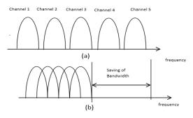
Fig.1.Comparison of (a) conventional multi-carrier technique and orthogonal multi-carrier modulation technique
