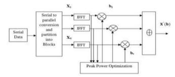
Fig.3. Block diagram of Partial Transmit Sequence
