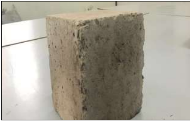
Fig-2 Fire affected concrete cube
