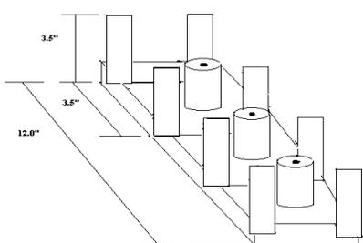
Figure no:-1 Fabricated Equipment to hold the sample
