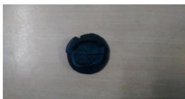
Fig No: 8 NBR-PVC Activated Carbon button
